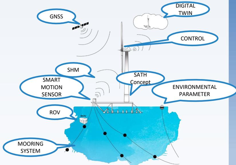
**Control algorithms** will be developed to take advantage of floating platform pose and mooring system condition information to optimize operation. Strategies such as blade pitch control, dynamic loading control and distribution of turbine operating thrust setpoints at farm level will be studied.
